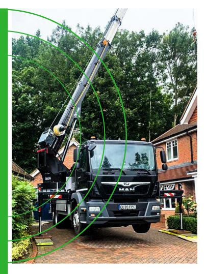
The operator can always have the best vantage point to safely operate the crane whilst it is lifting the load, this is due to the flexibility of the fact it is operated remotely by remote control, which can minimise the risk of blind lifting operations.
